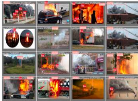
Our Machine Learning model detecting fire and smoke in various images
