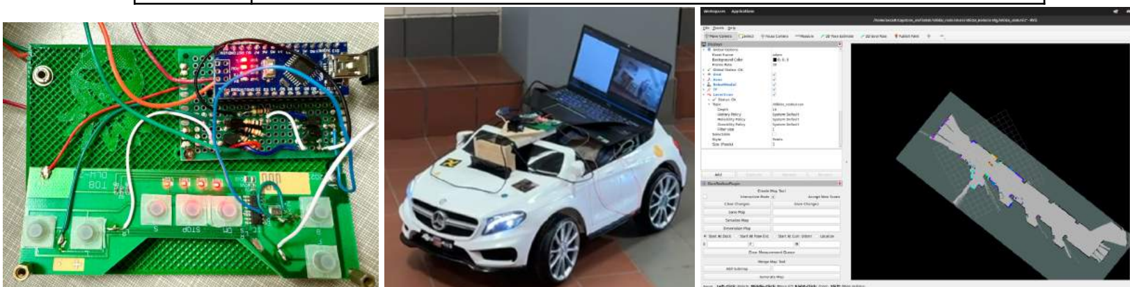
Fig. 1 (Left) Hacked RF controller with arduino nano
