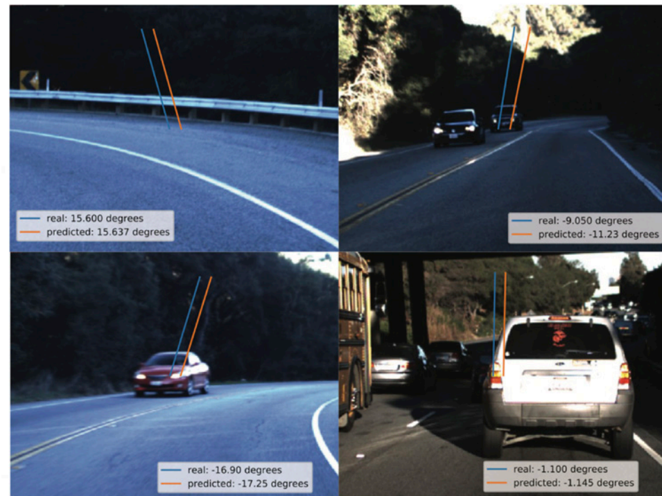
Examples of Steering Angle Prediction Using Dashcam video
